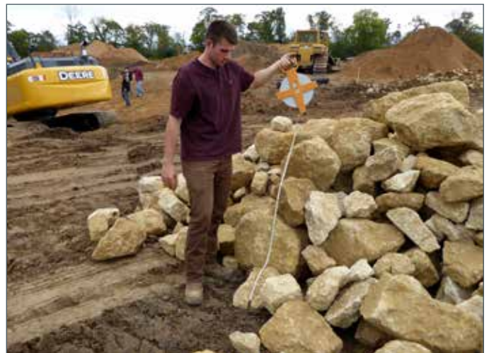
Jared Looney, Chippewa County Engineering Intern, measures gradation of limestone riprap
