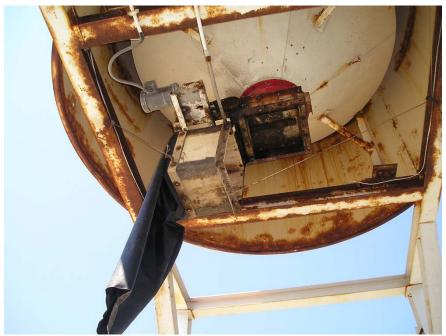
Although this set-up is on the bottom of a tower blender, the concept should be transferable to virtually any load-out. The "box" to which the "sock" is attached does not necessarily need to be as tall as shown.
