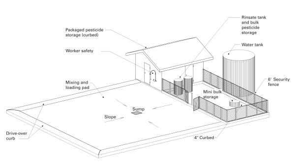
Figure 1.2. Small-scale facility, perspective view. Optional roof over entire facility.
