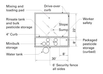
Figure 1.1. Small-scale facility, plan view. Optional roof over entire facility.
