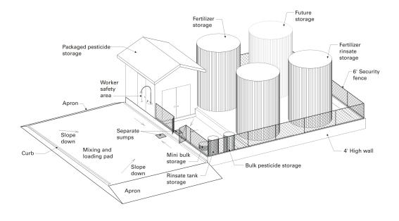
Figure 1.4. Medium-scale facility, perspective view. Optional roof over entire facility.
