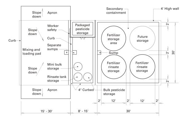
Figure 1.3. Medium-scale facility, plan view. Optional roof over entire facility.
