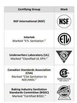
Equipment must be certified for sanitation by an ANSI-accredited program. This requirement applies to: sinks, refrigeration, hot-holding units, ice machines and cooking equipment. It does not apply to small appliances, such as microwave ovens and toasters.
