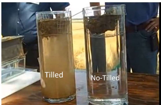
Figure 9 A rainfall simulation showing the differences in soil structure between tilled and no-till soil.
