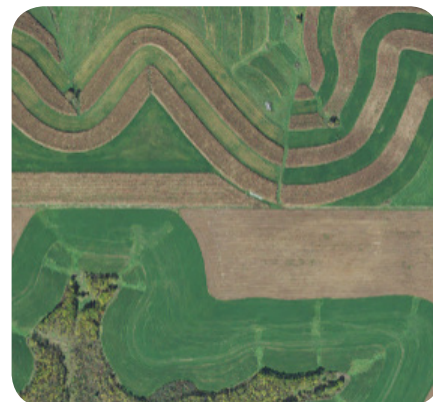
Figure 3. The top group of fields shows contour strip cropping with a grain and close grown crop on the width of the conservation planning length of slope. The bottom half of the aerial photo shows field contouring allowing for wider fields following the contour of the field.
