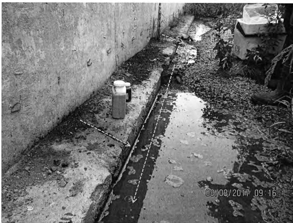
Photo 2: View of discharge points of leachate / process wastewater on the outer west wall of the feed storage bunker at the heifer site. Samples (LD1) were collected from the ponded wastewater adjacent to the location of the bottles. Dashed orange arrows indicate the direction of discharge flow. Photo direction is south and down.
