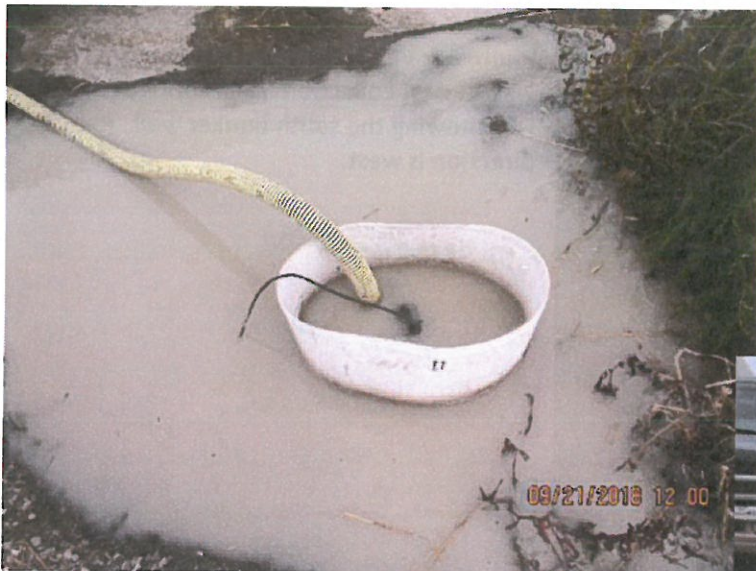
Photo 14 (left): Close up view of process wastewater ponded around the partially submerged plastic drum. Photo direction is down.
