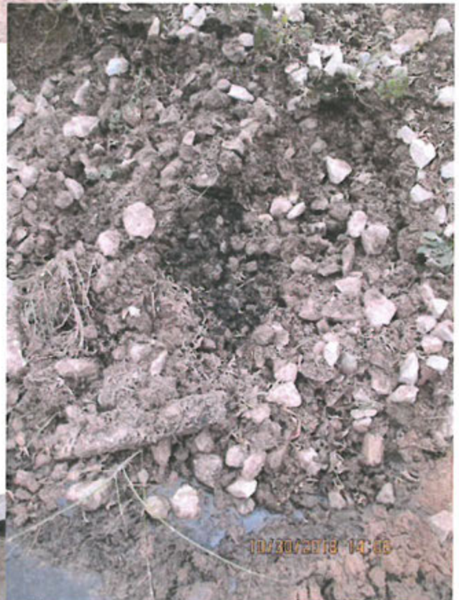
Photo 77 (right): Close up view of the stone, feed solids, and soil mixture piled against the exterior of the east wall of the FSA. Leachate seepage is visible. Photo direction is west and down.
