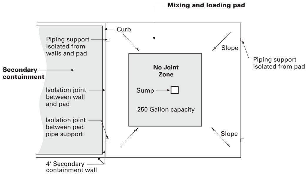
**Figure 5.8.** Common joints in mixing and loading pad (center sump design) Note location of piping supports.
