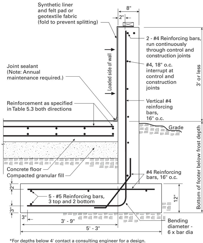
**Figure 5.7.** Frost wall for structural support of a synthetic liner.
