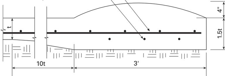
**Figure 5.3.** Concrete detail for mixing and loading pad floor with integral drive over curb. (See table 5.4 for concrete thickness, t).
