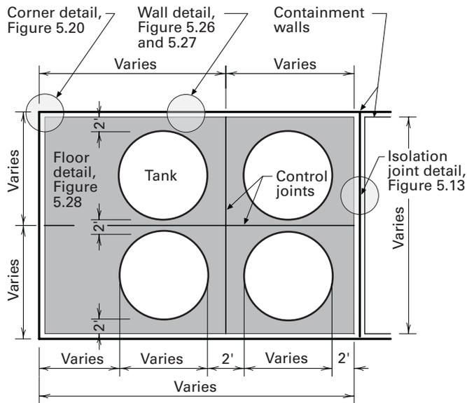
**Figure 5.11.** Common joints in secondary containment structure.
