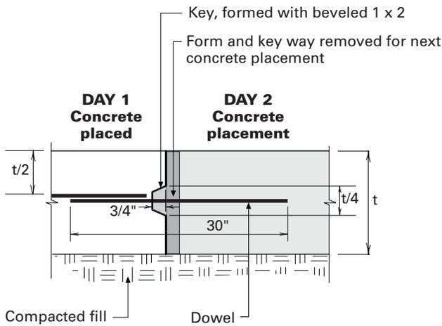
**Figure 5.14.** Construction joint.
