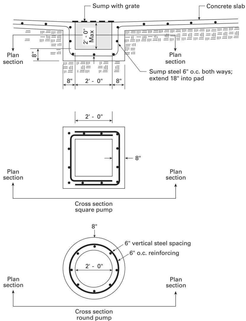
**Figure 5.5.** Sump or depression reinforcing schedule and design detail.
