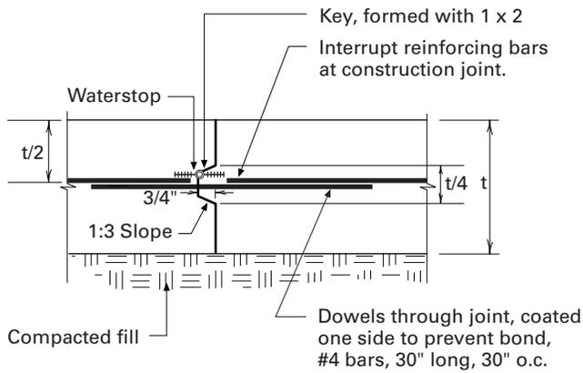
**Figure 5.24.** Floor construction joint with waterstop at midpoint (wet joint).
