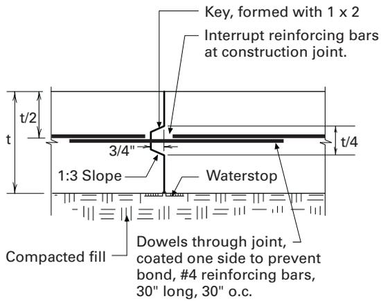
**Figure 5.25.** Floor construction joint with waterstop at bottom (wet joint).
