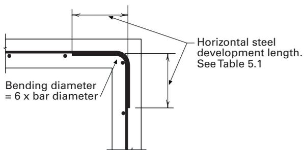
**Figure 5.20.** Reinforcing detail of a wall corner.
