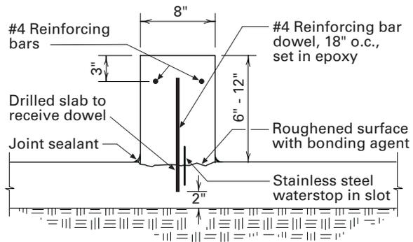
**Figure 5.19.** Retrofit curb-to-floor joint (dry or wet joint).
