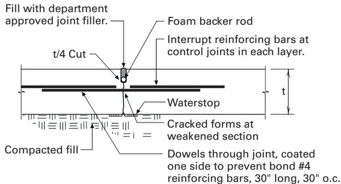
**Figure 5.22.** Floor sawn control joint with waterstop at bottom (wet joint).
