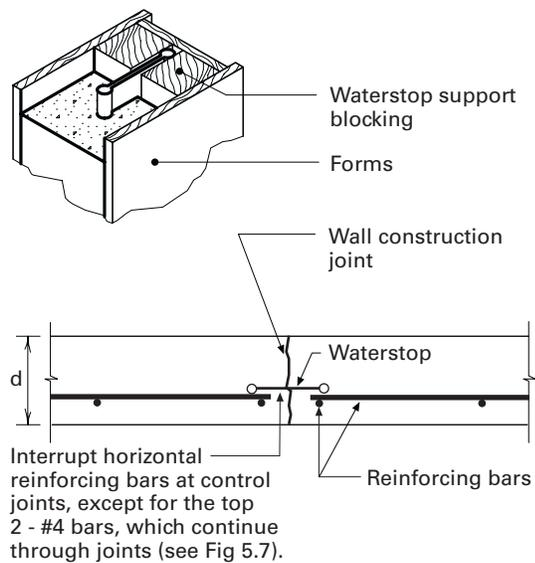
**Figure 5.29.** Wall construction joint with waterstop at midpoint of wall (wet joint).
