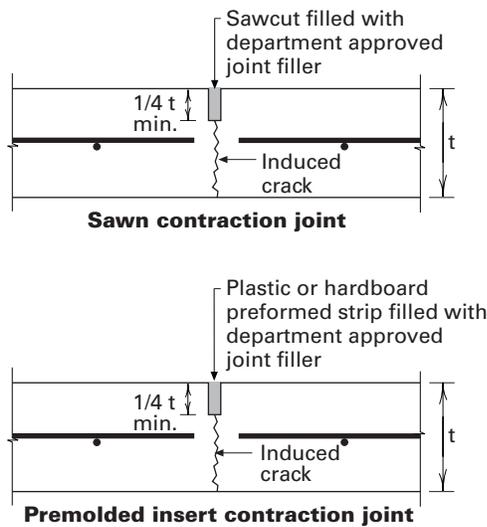
**Figure 5.15.** Control (contraction) joint.
