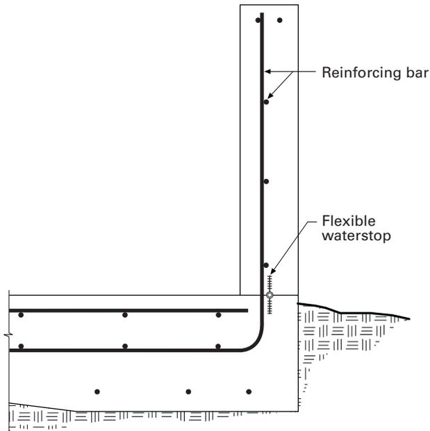
**Figure 5.16.** Wall-to-floor joint (wet joint).
