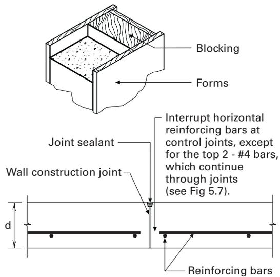
**Figure 5.28.** Wall construction joint (dry joint).
