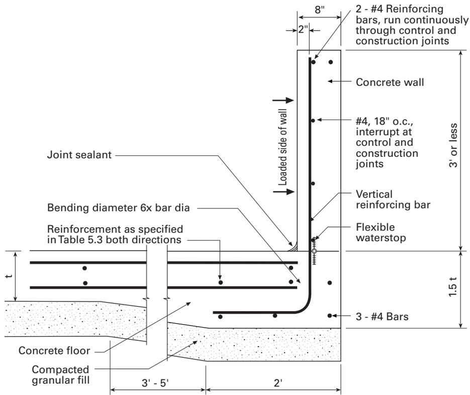
**Figure 5.6.** Reinforcing schedule and design detail for secondary containment wall.
