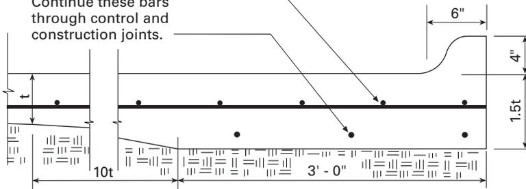
**Figure 5.4.** Concrete detail for mixing and loading pad floor with integral edge curb. (See table 5.4 for concrete thickness, t).
