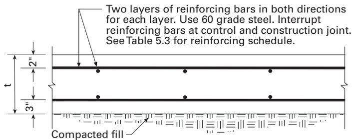
**Figure 5.1.** Concrete detail for secondary containment floor with two layers of reinforcing. (See table 5.2 for concrete thickness, t).
