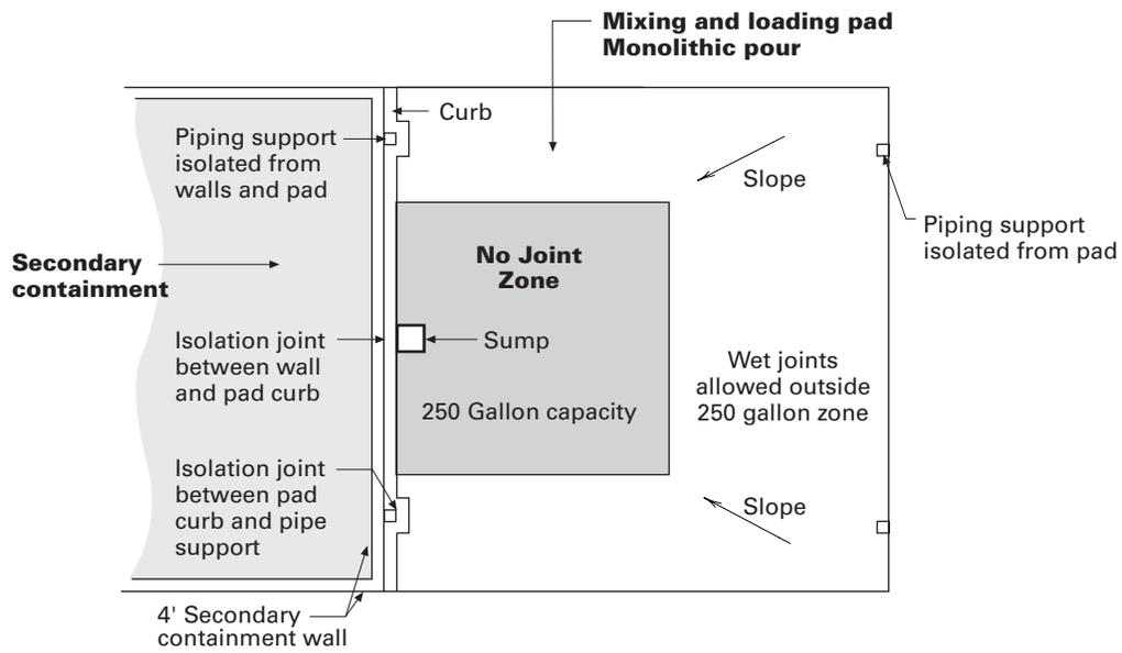
**Figure 5.10.** Common Joints in mixing and loading pad (side sump design).
