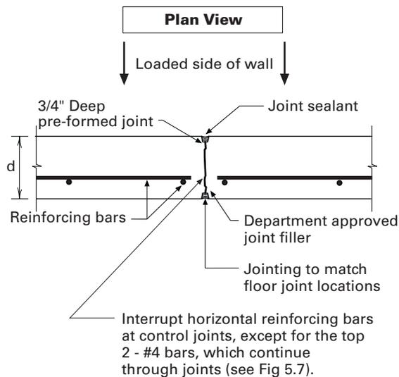
**Figure 5.26.** Wall sawn or formed control joint with joint filler (dry joint).
