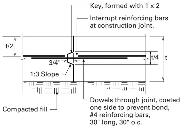
**Figure 5.23.** Floor construction joint (dry joint).
