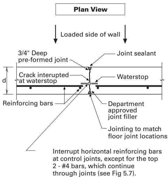
**Figure 5.27.** Wall sawn or formed control joint with waterstop at midpoint of wall (wet joint).
