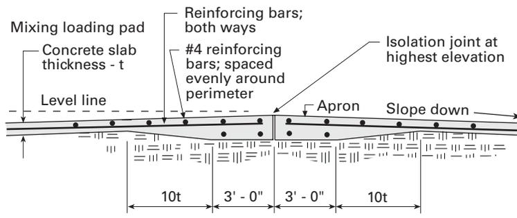
**Figure 5.30.** Floor Isolation joint (dry joint).
