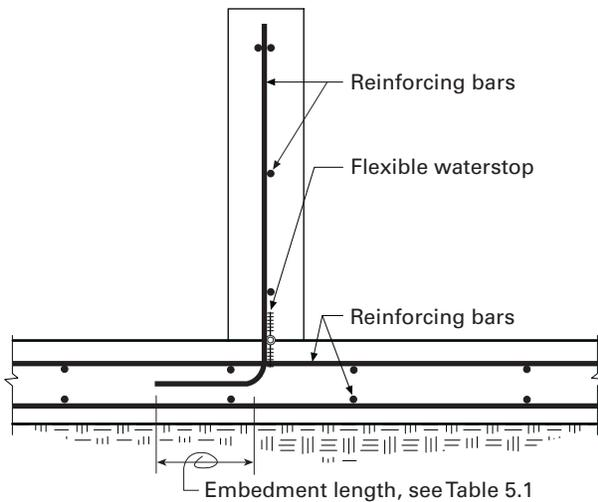
**Figure 5.17.** Interior wall-to-floor joint (wet joint).
