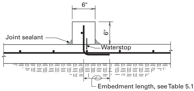
**Figure 5.18.** Interior curb-to-floor joint (wet joint).
