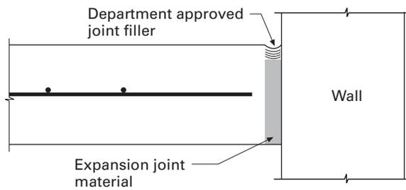
**Figure 5.13.** Isolation joint.
