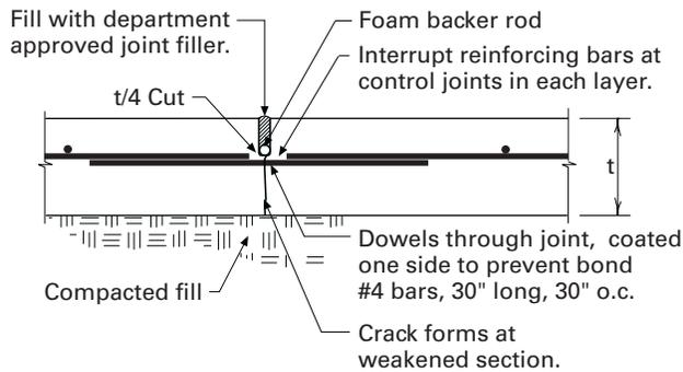
**Figure 5.21.** Floor sawn control joint with joint filler (dry joint).
