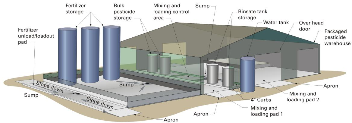
**Figure 1.6.** Large-scale facility, perspective view. Optional roof over entire facility except fertilizer secondary containment and bulk unload pad.
