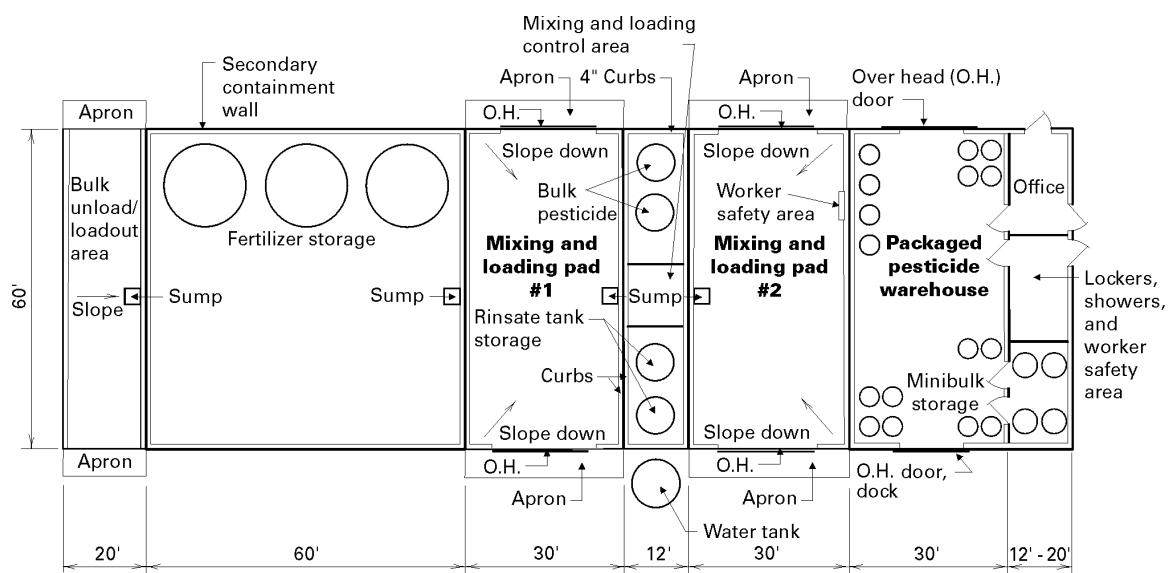
**Figure 1.5.** Large-scale facility, plan view. Optional roof over entire facility except fertilizer secondary containment and bulk unload pad.
