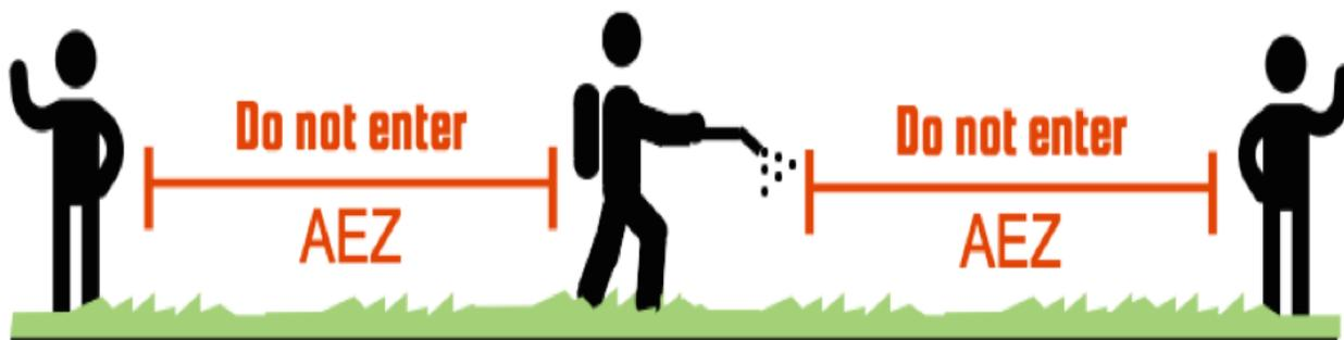
The AEZ is measured as a horizontal straight line from the application. It moves with the equipment and surrounds the application equipment in all directions, like a halo. If the equipment moves, the AEZ moves as well.
