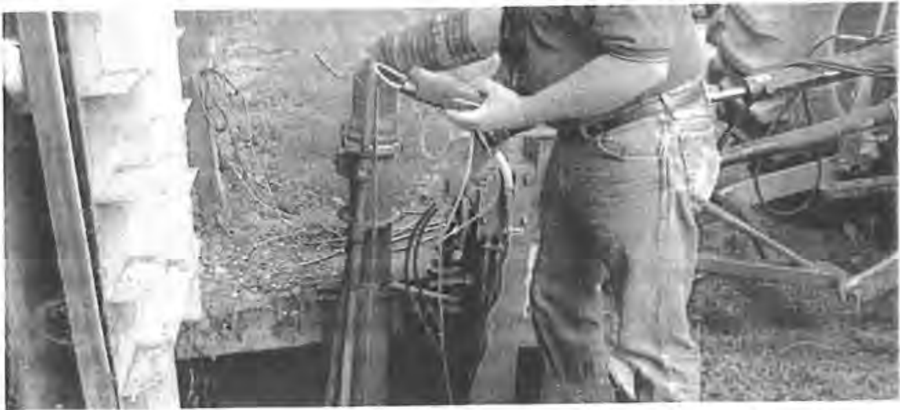
Figure 4. Always remain outside the manure storage facility when taking initial gas measurements.
