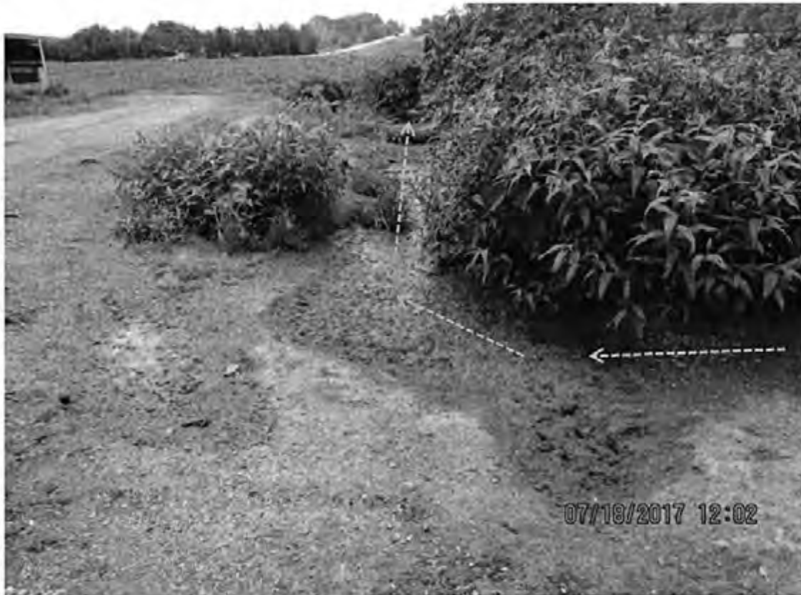
Photo 71: Close up view of leachate discharging from the south wall of the feed storage area at the heifer site. Orange dashed arrows indicate flow direction of leachate. Photo direction is south.
