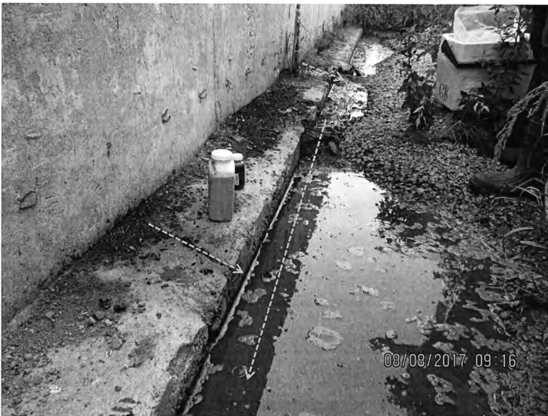
Photo 2: View of discharge points of leachate / process wastewater on the outer west wall of the feed storage bunker at the heifer site. Samples (LD1) were collected from the ponded wastewater adjacent to the location of the bottles. Dashed orange arrows indicate the direction of discharge flow. Photo direction is south and down.
