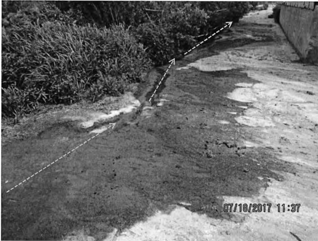
Photo 46: View of the leachate discharge path as it flows NE from the NE corner of the feed storage area. Orange dashed arrows indicate the flow path and direction of leachate. Photo direction is east and down.
