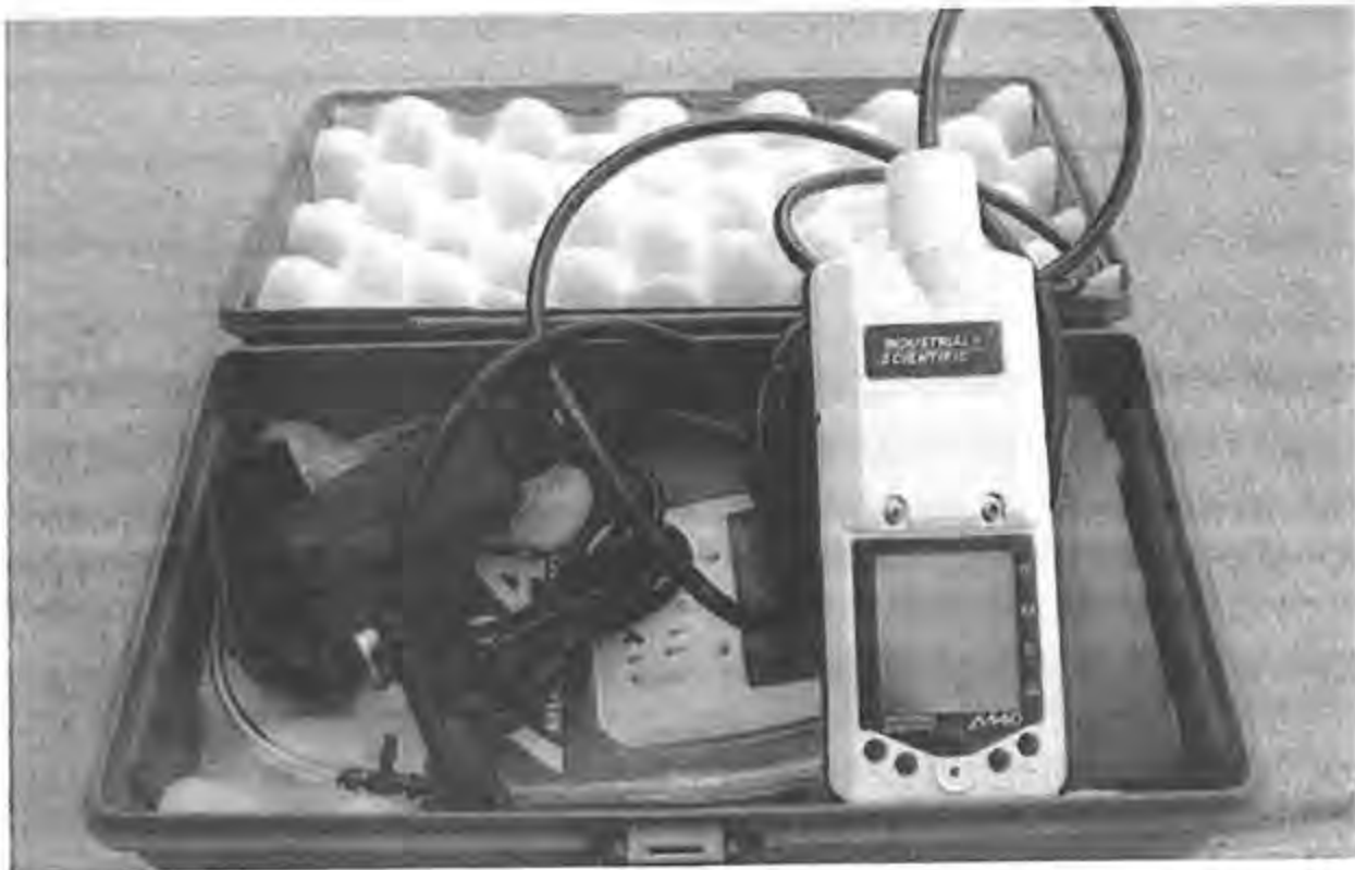
Figure 3. Hand-held, portable multi-gas monitors measure most of the manure gases and oxygen levels.
