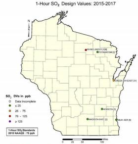
Figure 29. The 1-hr  $SO_2$  design values for each monitoring site for 2015-2017.
