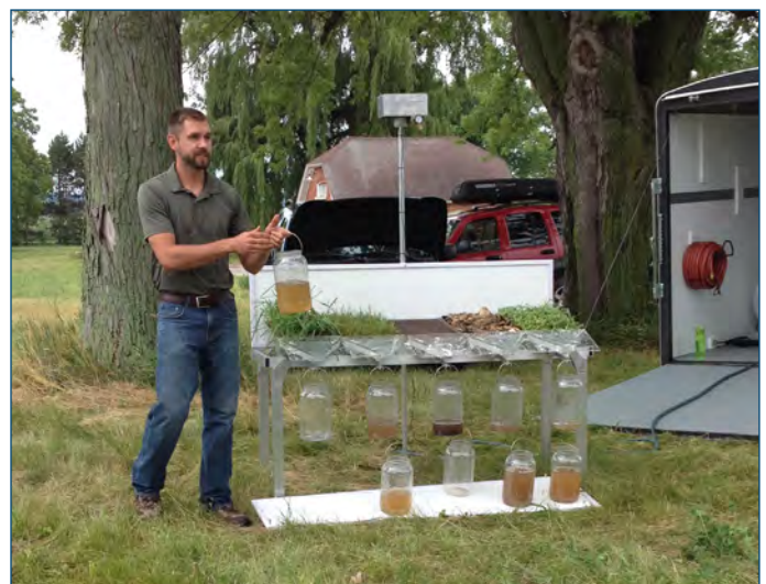
Aaron Pape, Sauk County’s former education coordinator, uses the county’s new rainfall simulator to demonstrate how good cover and healthy soil can protect both land and water.
